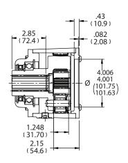
OUTPUT SHAFT ROTATION SAME AS MOTOR SHAFT ROTATION
